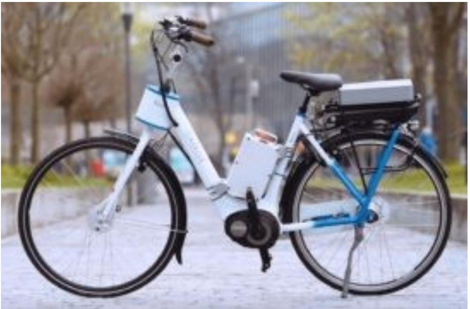
Steer assist system prototype
