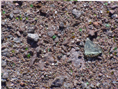
Coarse green glass particles with occasional large pieces
